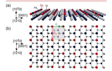
Figure 3. Perspective view of a ball model of the idealized, long-range, chemical ordering of the two-dimensional monolayer shell on the InAs sidewall facet, based on the ordering and antiordering vectors extracted from pair correlation function. (a) Side and (b) top view with surface unit cell (gray shaded area) and ordering as well as antiordering vectors shown as green and red arrows, respectively.
